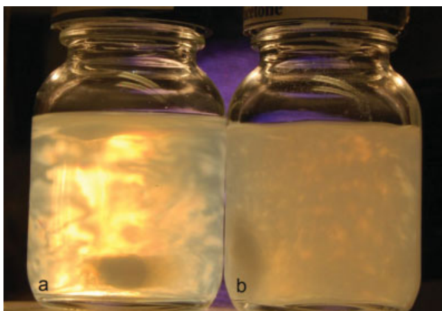
Figure 1 Photographs showing the flow birefringence of whiskers in (a) water and (b) acetone. [Color figure can be viewed in the online issue, which is available at www.interscience.wiley.com .]
